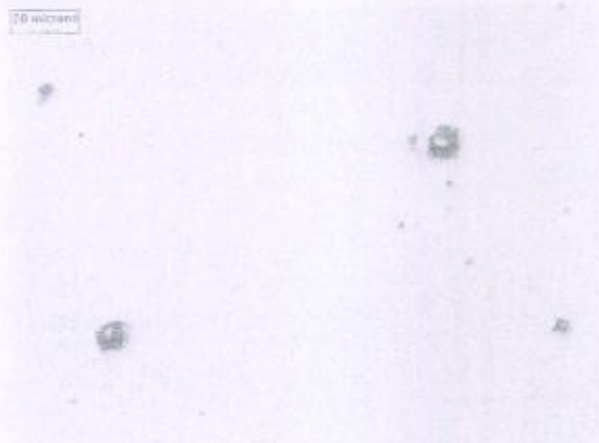
Fig. 2-Hexachloroethane Degassed. Lot of inclusions and porosities observed.
